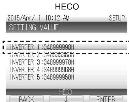
④ The parameter menu will appear. (See Page 29 for a description of the parameters in the parameter menu.) Scroll through the parameter menu using the [↓] button. To select a parameter, press the [ENTER] button.
